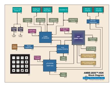
The AMBE-20x0™ HDK is able to demonstrate the capabilities and benefits of the AMBE-2000™ / AMBE-2020™ low-bit-rate vocoder in real-time, without investing in engineering design and hardware development. Two AMBE-20x0™ HDK vocoder boards may be connected together to easily establish a full-duplex (encoding and decoding) low bandwidth voice compression communication system.
